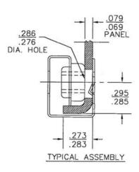
**G NUTS** combine the high strength of a multithreaded nut and spring steel while eliminating the need for multiple tapped holes.
