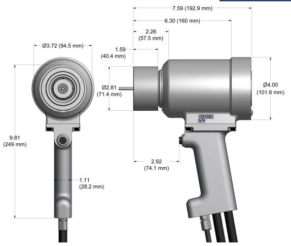
The **GB3585** and the **GB3585A** are hydraulic installation tools designed specifically for the efficient installation of 1/2" - 3/4" diameter pintail and pintail-less style lockbolts. It weighs just over 19 lbs. (18.6 kg). and can be operated in any position. It has a 1.810" (46 mm) fastener stroke and a rated pull load of 45,668 lbs. (203 kN) @ 7,400 psi. (510 bar).
